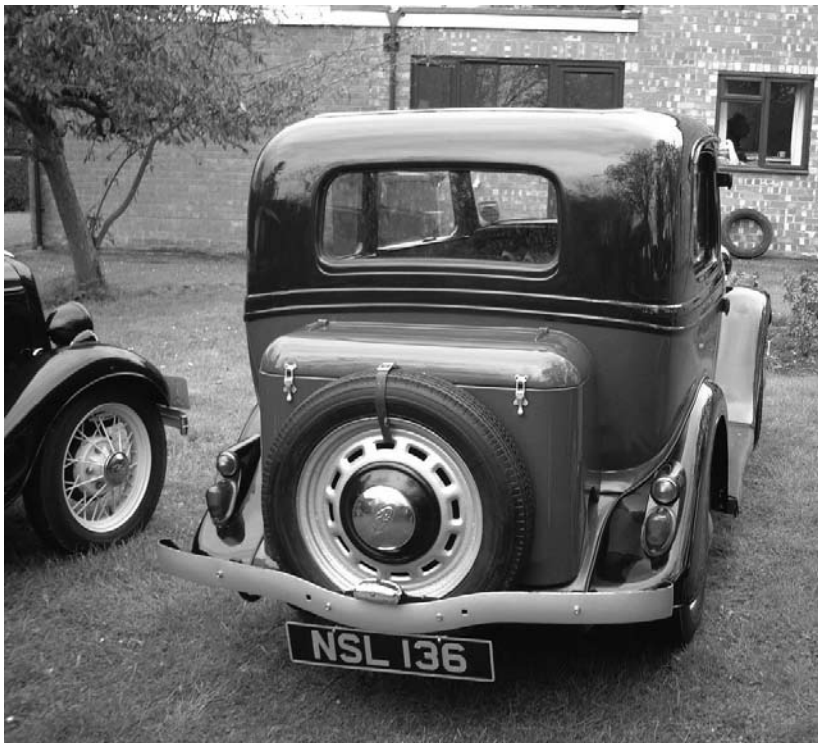
Richard Coleman's recently acquired Tudor model "Y" showing the added boot and the pressed steel spare wheel which is replicated on each of the axles.
