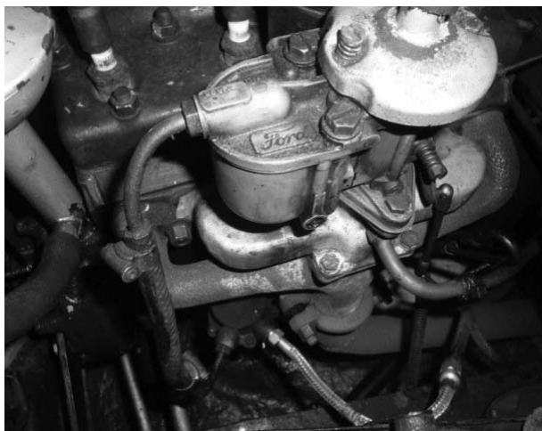
Billy's carburettor with an extra flexible pipe to the fuel pump.
