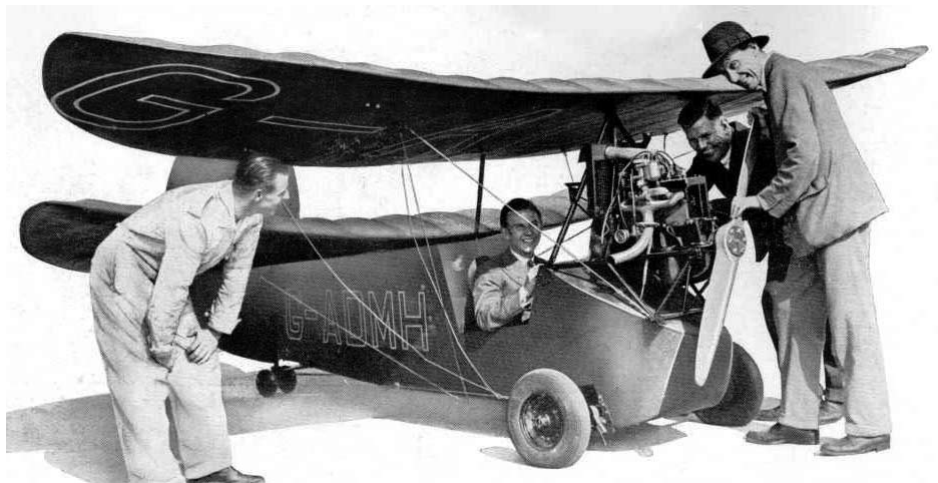
The Flying Flea home-built light aircraft clearly showing the Model "C" engine power-house.
