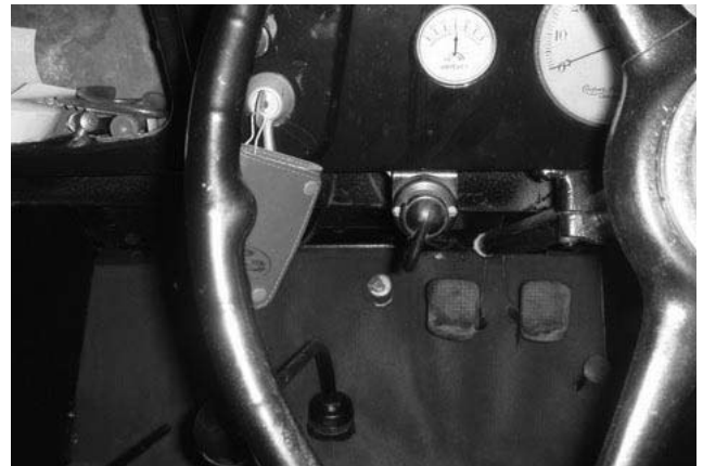
The dashboard of one of Dave Ball's De Luxe Fordor ex-Brighton taxis showing the location of the trafficator switch.
