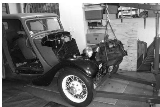
Out with the 8 hp engine ....2. ... and in with the 10 hp. Note the four-bladed fan, which was fitted to many export models. David's Fordor flying the flag at the Christchurch annual swap meet in October
