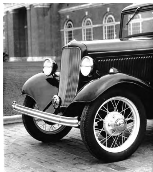
One of the 14 Prototypes at the rear of the Henry Ford Museum in Dearborn (then called The Edison Institute) in January 1932, just prior to shipping to Dagenham (see also the back cover of this issue). Note the Ralph Roberts curved 'shovel' base design input to the radiator grille, which was not repeated on the Gregorie-designed production body.
