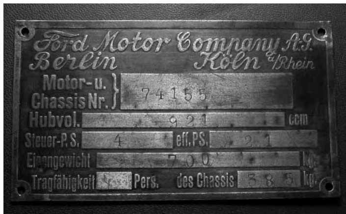
A similar manufacturer's plaque to that on Harold's bulkhead. However, note that this one, belonging to Y74155 (manufactured August 1934) shows a weight of 700 Kg.
