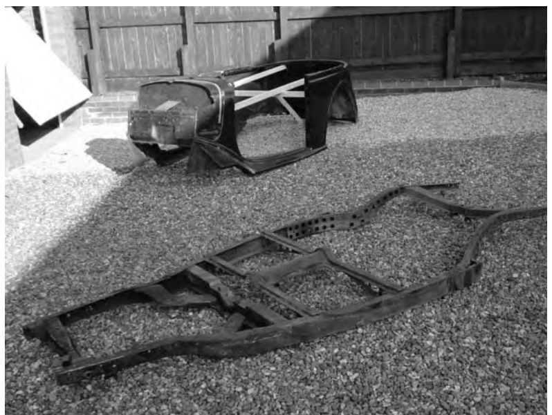
"Body & chassis no longer close friends. Note bracing of body. See also page 27"
