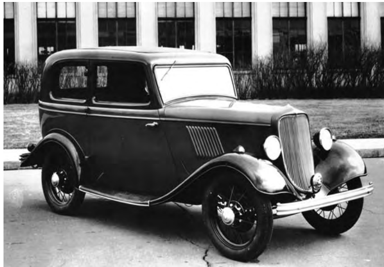
The green and black pre-production Model 19 ready for shipment to England outside the Ford Engineering Laboratory in Dearborn on 16 th March 1932. Note the distinguishing ten bonnet louvers and the Model "A" door handles.
