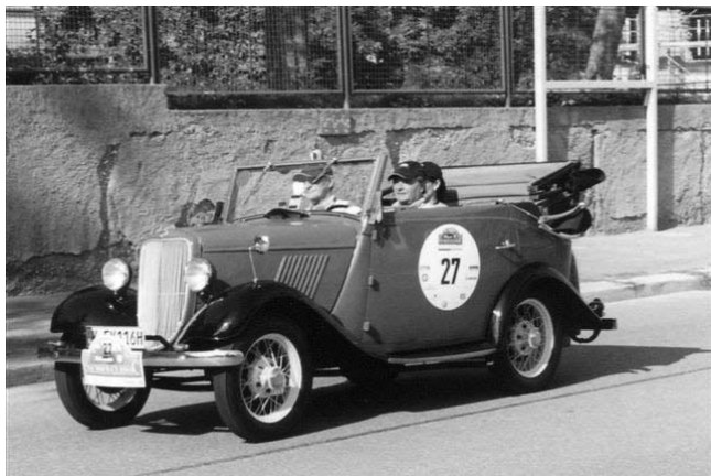
A surviving Deutsch bodied Köln cabriolet. Note that this body has running boards, unlike the cabrio-limousines and limousines (saloons), which did not, but had mud flaps to the rear of the front wings.
