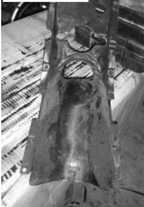
The gearbox/propshaft tunnel showing, at top right, the hole into which the dip switch is fitted.
