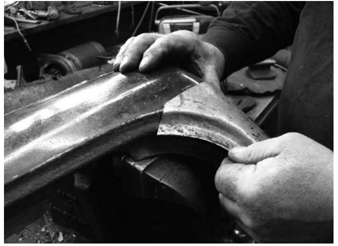
New panel bits, skilfully made and welded in – here the top of the windscreen surround
