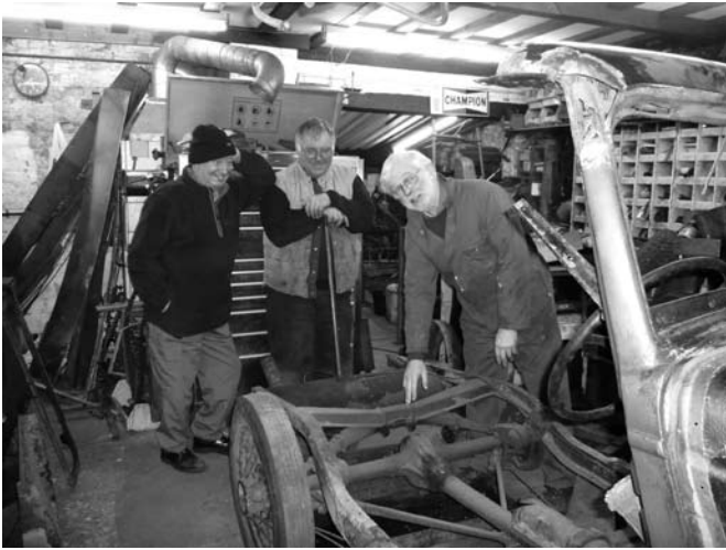
Bob explains the procedure for removing the rear axle to the delight of Noel and Roger. Although not obvious from this photograph, the van rear spring has an extra leaf to support the extra loading
