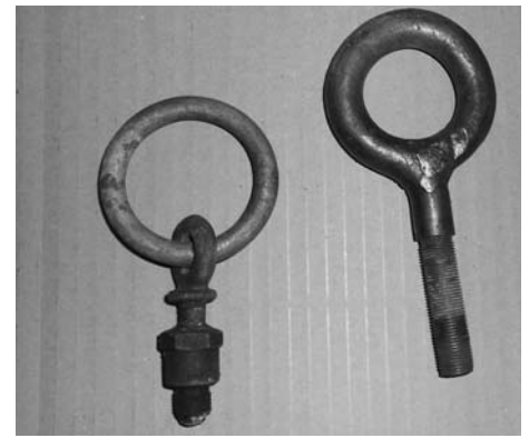
Two examples of a simple engine lifting tool: either a hand-crafted tool, or one made from the base of a spark-plug, the latter is more prone to scrutiny by the ‘Elf & Safety’ chap-pees.”
