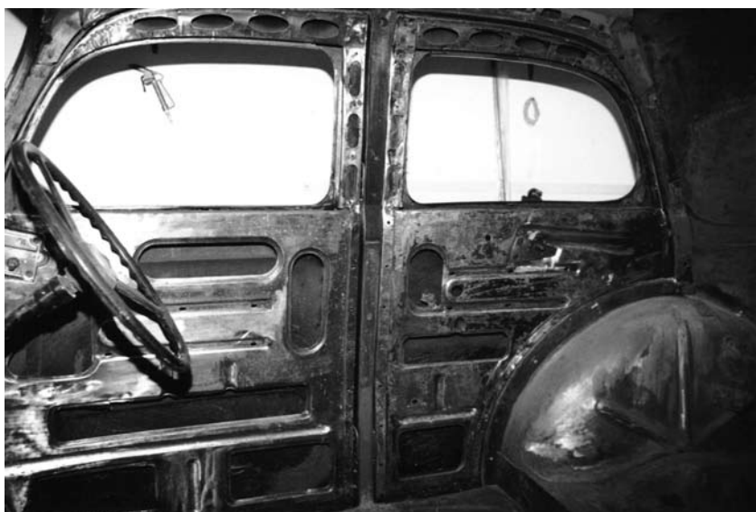
The pressed steel inner door and body panels of John Keenan's Model "C" during its restoration in 1992
