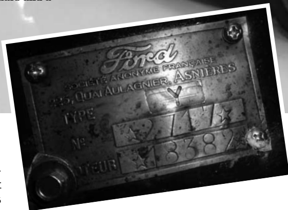
The Ford Asnières assembly plant plate attached to the bulkhead of the Kelsch (No. 2717), demonstrating that the bodies arrived with chassis at the Asnières plant before assembly.
