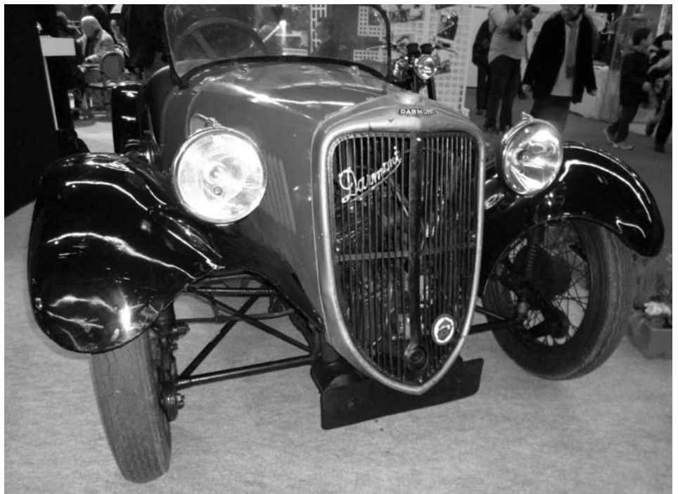
Above: The front grille showing the air-cooled twin cylinder engine behind and the 'filler' cap on top.
