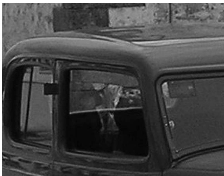
A close-up of the roof above the doors without rain guttering and with the heavy overhang over the windscreen.
