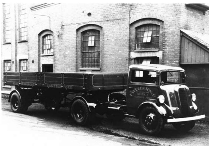
1939. The 7V range extended to include four and five ton models and a County Commercial Cars' six-wheel conversion based on the five ton chassis. The six-wheeler and the tractor unit increased the payload to six tons.
