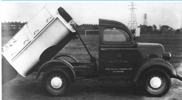
Using the 1172cc (old 24hp) four cylinder engine from the 10hp car. Offered as a van or chassis with open back cab, both models had a conventional channel chassis with transverse leaf springs front and rear. In production for nineteen years as a van and with every conceivable type of purpose-built bodywork.
