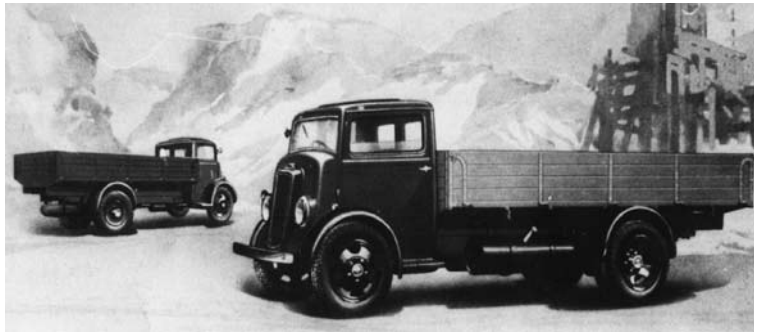
1934. BBE two-ton range 30hp V8 engines, fully forward control cab and available as a truck or van. In 1935, a six-wheel 'Surrey' conversion by County Commercial Cars Ltd. gave a six ton payload.
