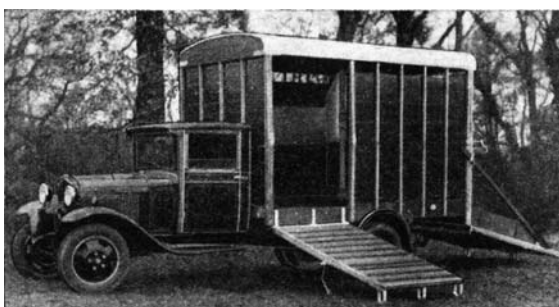
1932. The two and three ton normal control 24hp BB range offered two-wheelbases and, in 1935, a six-wheel model with a 30hp V8 engine.
