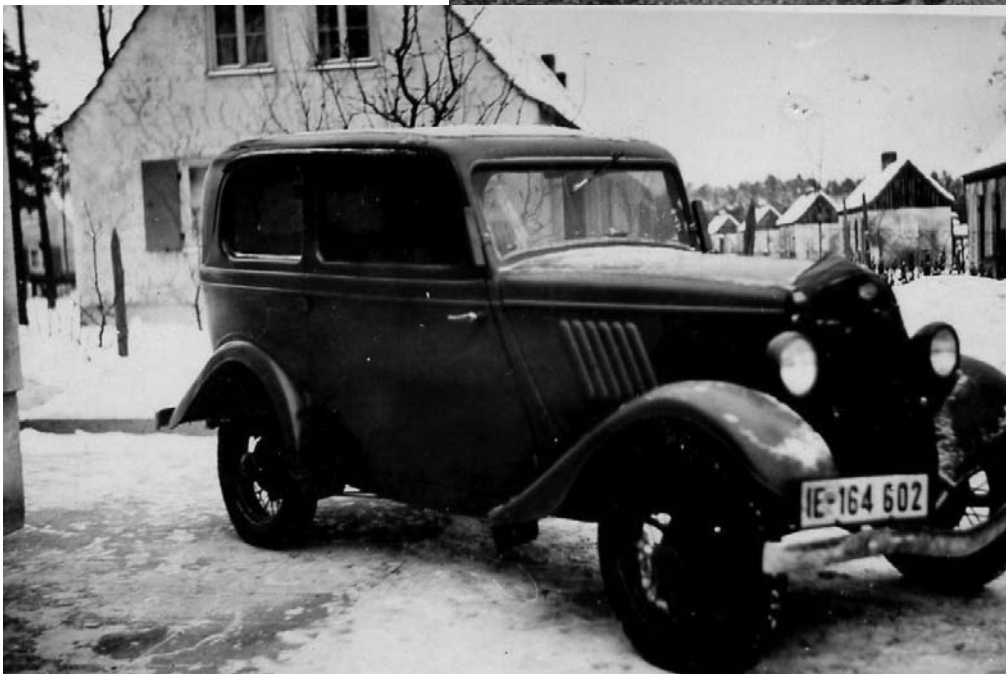
A 1936 Köln in a wintry scene in Brandenburg Province, Germany, in 1942. Note no running boards or groove in the bumper and mud-flaps – standard Ford Köln features.
