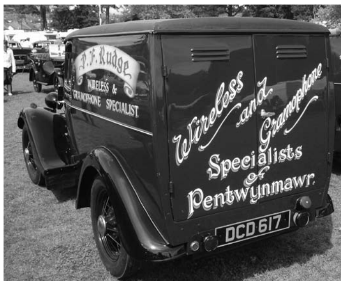
Paul Rudge's January 1937 van showing its present-day livery. Note the original three louvred rear doors, the mud flaps in lieu of running boards and (incorrectly) the lack of a spare wheel on the near-side – the spare was moved from the driver's door in October 1935 in production.
