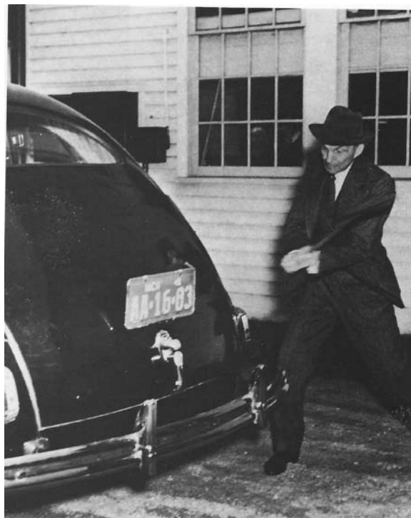
Henry Ford smashing the soya panel with the back of an axe-head, proving the strength of the material
