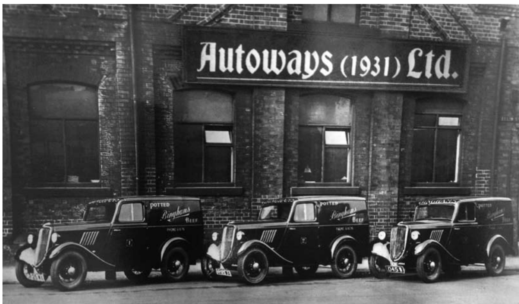
Three Model "Y" vans, on trade plates, waiting delivery from Autoways in Sheffield. Note that the long rad vans do not have bumpers and have their spare wheels on the drivers' doors, i.e., manufactured before October 1936.
