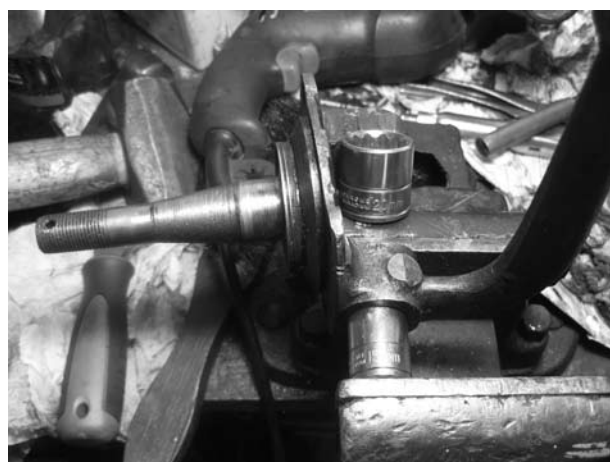
"Stub axle with new bush having been partially inserted using a 20mm socket and hammer, now held in the bench vice with the bush fully inserted using 15mm socket."
