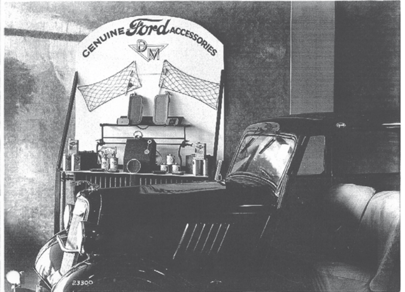
"A display of Ford accessories at Dagenham Motors Ltd., the main Ford dealer off Oxford Street in London. Note the additional accessories on the car in front of the stand. It is a two-door (Tudor) with sliding roof, probably from 1935/36. Its additions include trafficators, a second (slaved) windscreen wiper, a racing greyhound bonnet mascot (probably from a Model 40 V8 Greyhound), an abbreviated radiator muff, which covers only the radiator grille, a badge bar and headlamps with unusual rims!"
