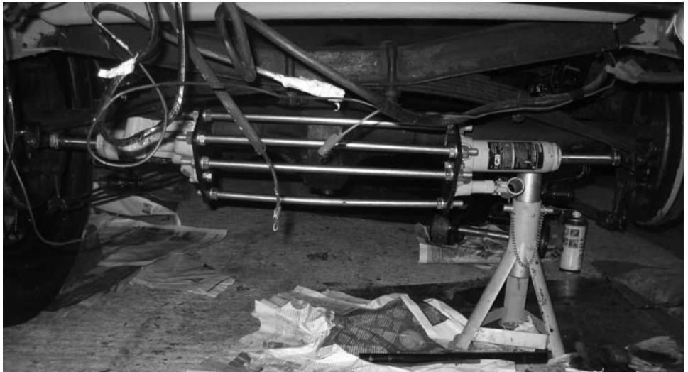
The rather elaborate spring spreader that John inherited from his father. It allows space to accommodate the differential housing in the same way as the standard Churchill spreader.
