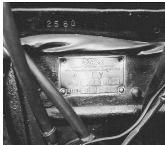
An Asnières plaque as it appears on the French Model "Y"s. Note this belongs to Y19835 and was the 2580th car to be assembled in the Ford plant.
