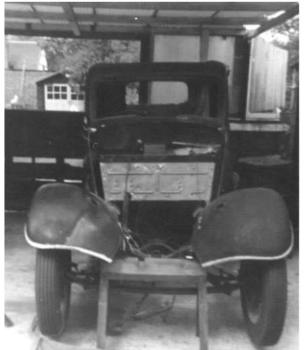
APP 625 back home on all four wheels, some work done but a long way to go, still has the remains of white paint on the wings that I believe was common during the war years when the use of lights was forbidden.
