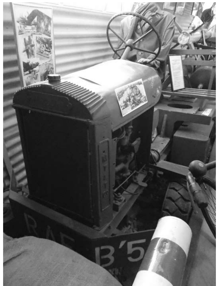
Bomb tractor fitted with Ford 8HP engine and B&W Governor
