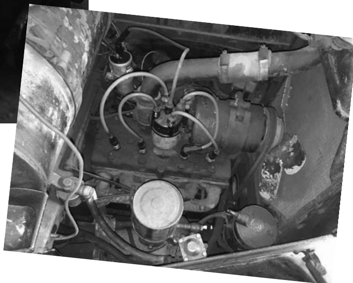
Under the Belilla's bonnet, we see that the petrol is gravity fed from a large tank in front of the scuttle, reminiscent of the Model "Y" prototype. Photographs courtesy Karl Dillon.
