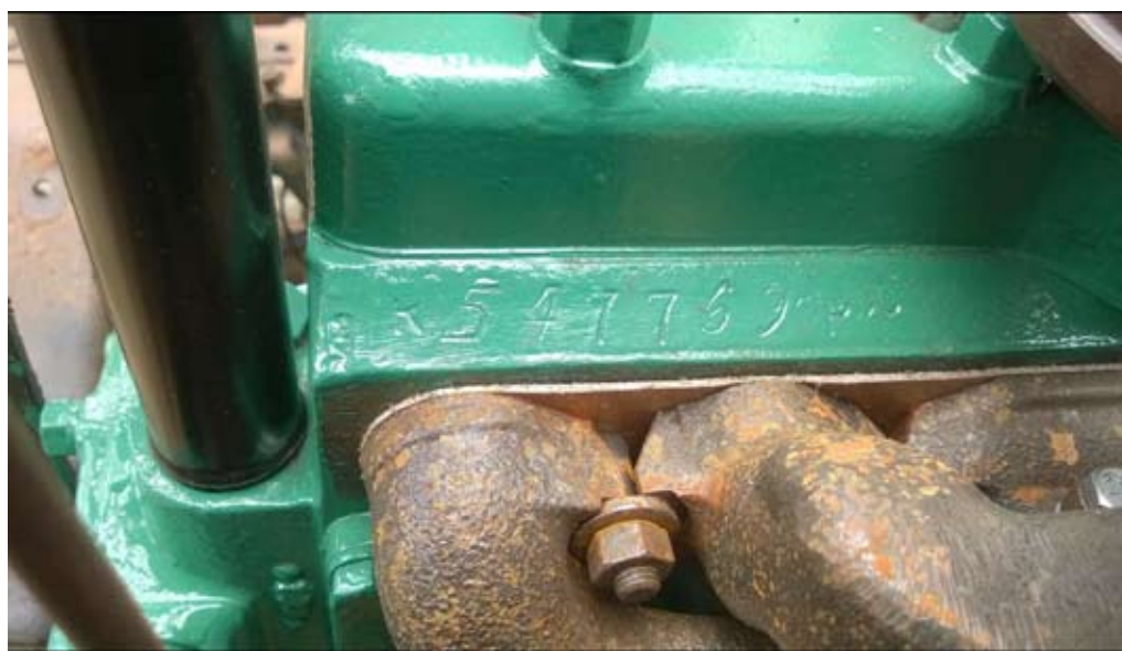
The overhauled engine number, which, surprisingly, does not indicate whether it is an 8 h.p. (Y) or 10 h.p. (C) following the R at the start. It does however have a 'P' and a 'C' following the number indicating that the engine can be used for Passenger or Commercial vehicle use for road tax purposes.
