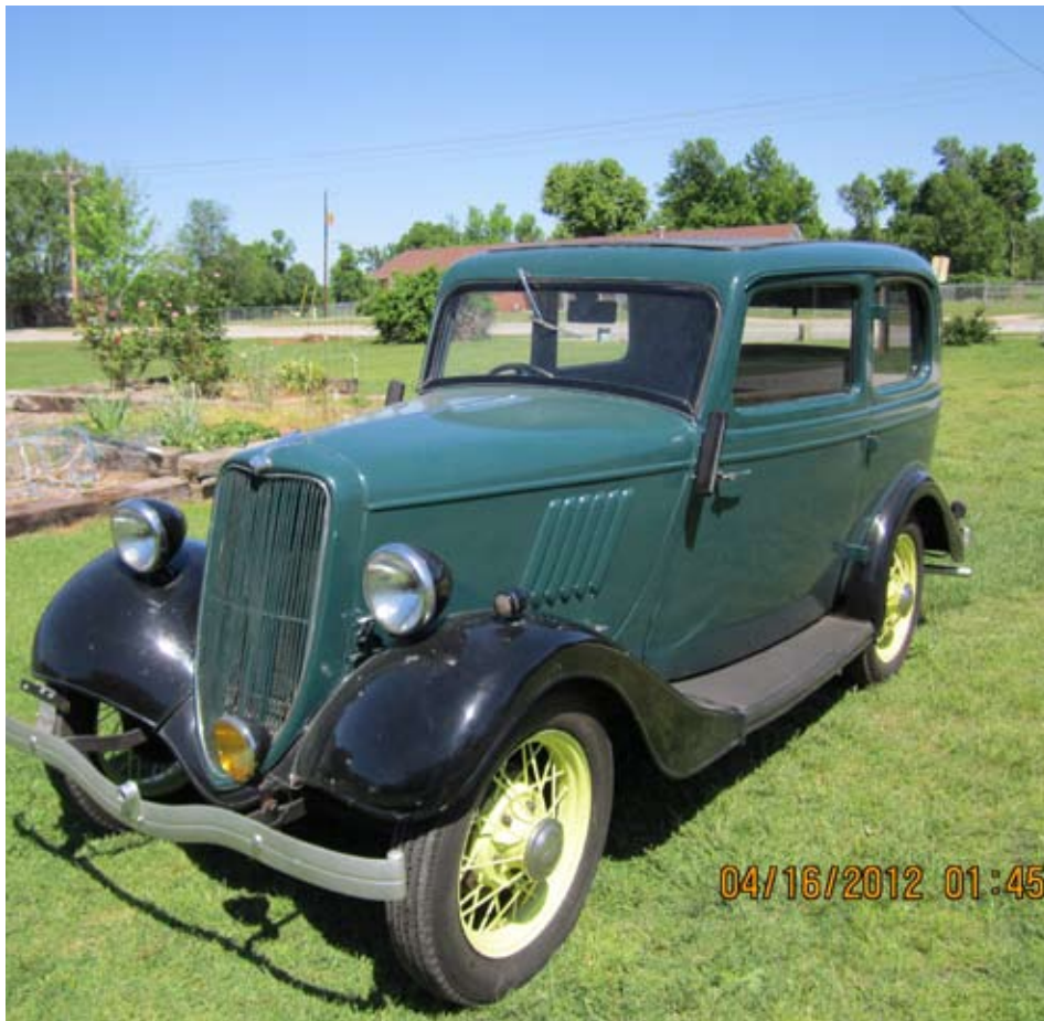
Y157501 photographed in Arkansas in 2012. Note the odd sidelights and the add-on starter dog in the centre of the front bumper
