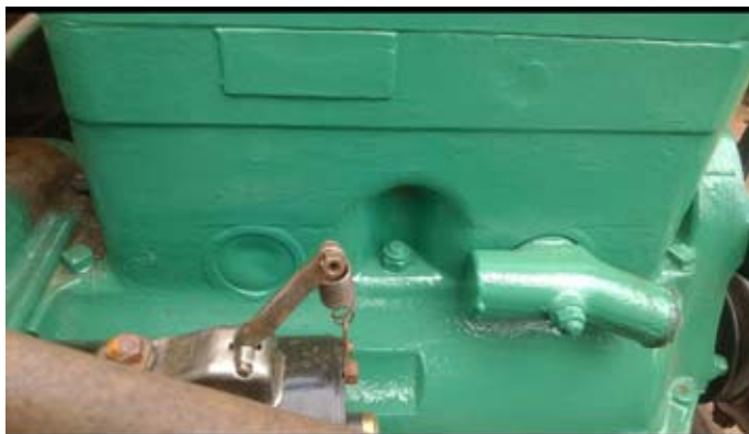
The water inlet to the marine engine showing the blanked off second hole. As the water would have been pumped through the engine, only one inlet was necessary.
