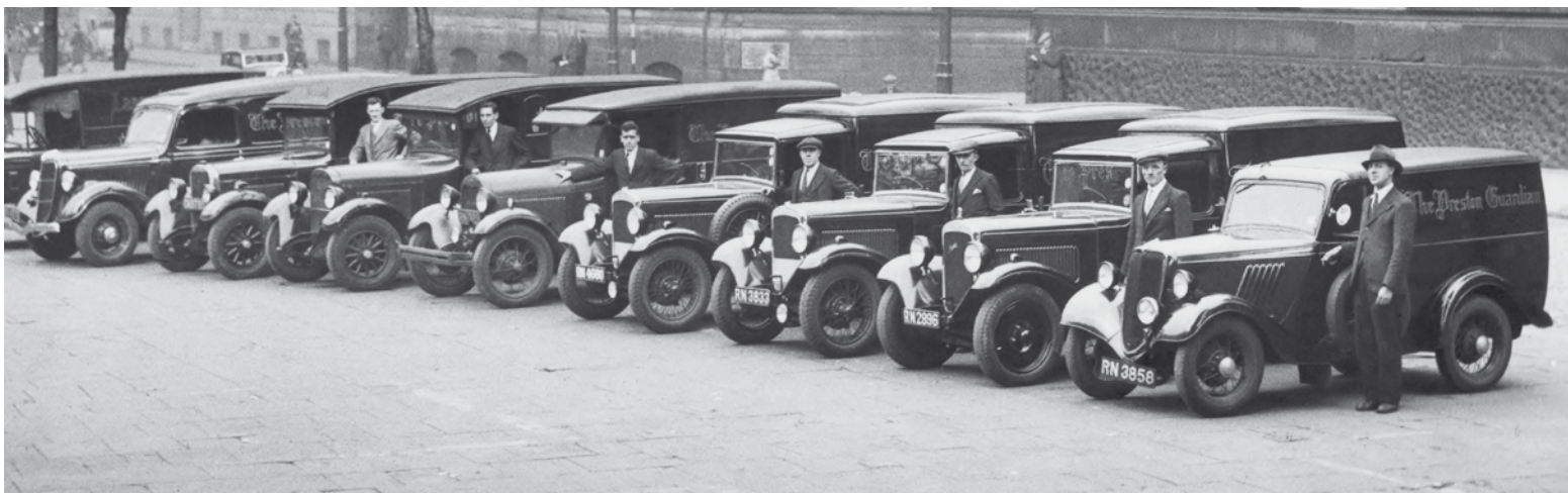
The Preston Guardian van fleet goes up market with the first streamlined mass produced vans. Note the upright windscreens except for the V8 Model 48 van at the far end and the 1935 Model "Y" van at this end. The sun's reflection says it all!"
