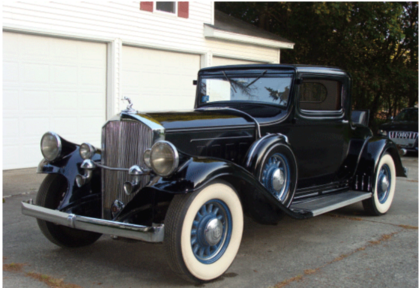
A 1930 Pierce Arrow distinctly showing the faired-in headlamps.
