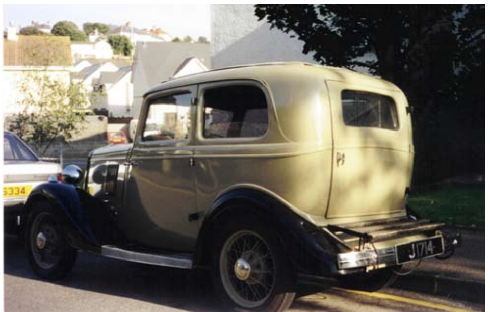
The Jennings conversion on the Model “Y” showing the goods access door at the rear.
