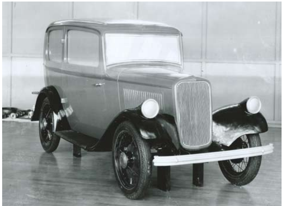
An early clay model study for the Model 19, probably designed by Jo Galamb. Note the faired-in headlamps. This concept was probably rejected on the grounds of difficulty in pressing out the wings in mass-production quantities.
