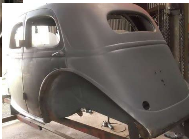
The rear body tub of Bill’s ute now ready to be wood-lined.
